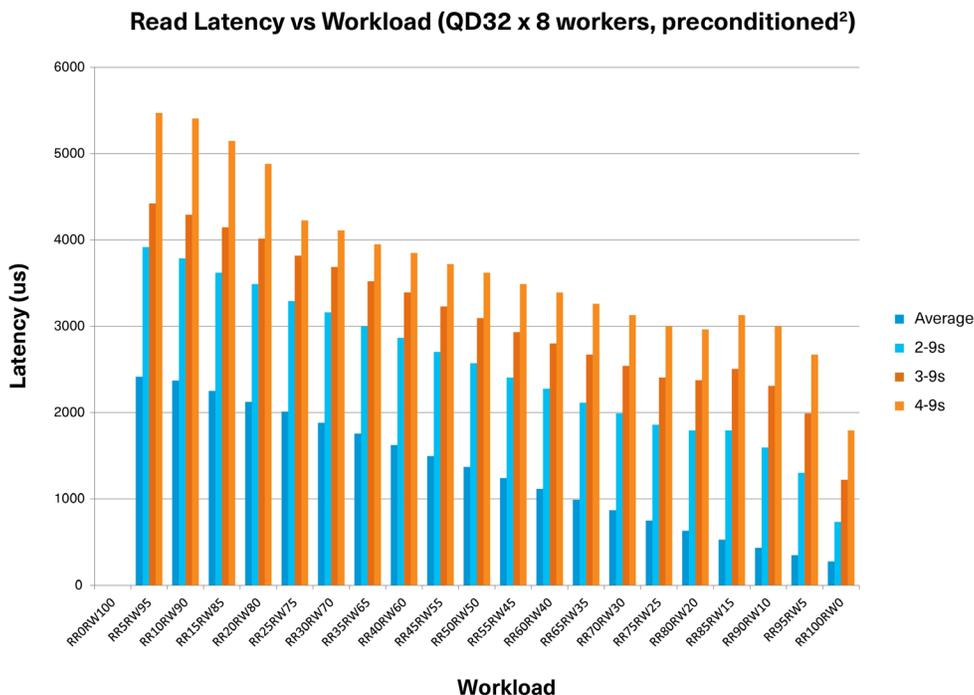
Figure 2: XD6 Series read latency on mixed workloads
