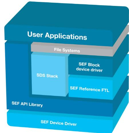
Figure 1: Software-Enabled Flash host software block diagram
