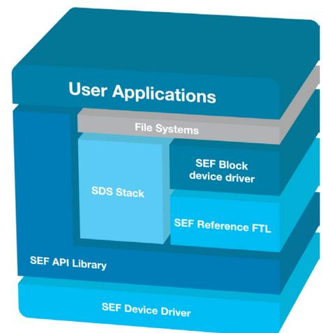
Figure 3: Software-Enabled Flash technology host software block diagram
