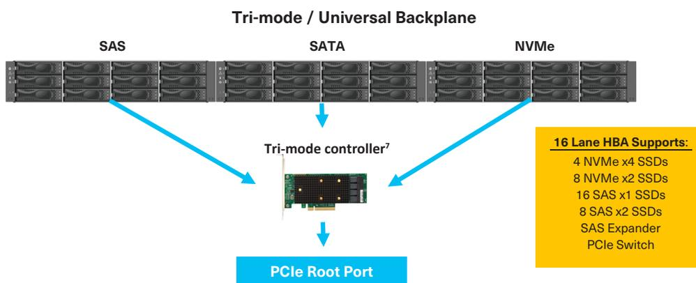
Figure 1: The U.3 tri-mode universal storage configuration for SAS, SATA and NVMe protocols
