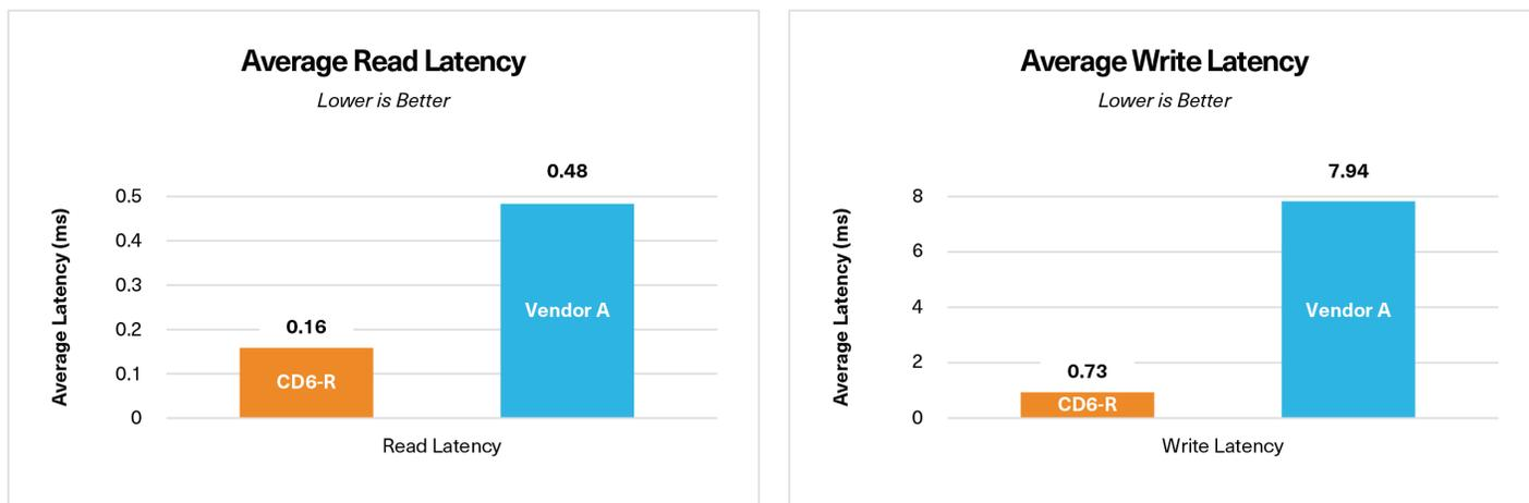
Figure 2: Latency comparison of data center PCIe 4.0 vs PCIe 3.0 NVMe SSDs (lower is better)
