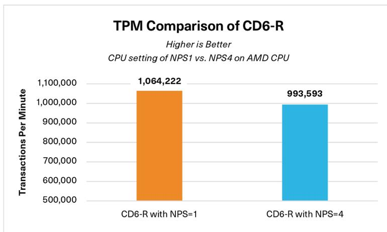
Figure 4: TPM comparison of CD6 Series PCIe 4.0 NVMe SSDs with the CPU setting at '1' and '4' (higher is better)
